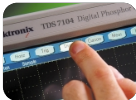
► Figure 61. Touch-sensitive display naturally solves issues with cluttered benches and carts, while providing access to clear, on-screen buttons.
