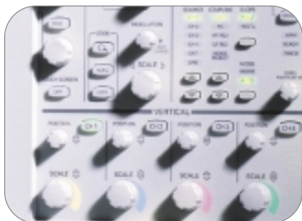
► Figure 60. Traditional, analog-style knobs control position, scale, intensity, etc. – precisely as you would expect.
